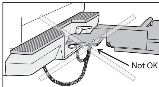
binding; however, note that excessive slack will allow the chains/cables to drag on the ground.
