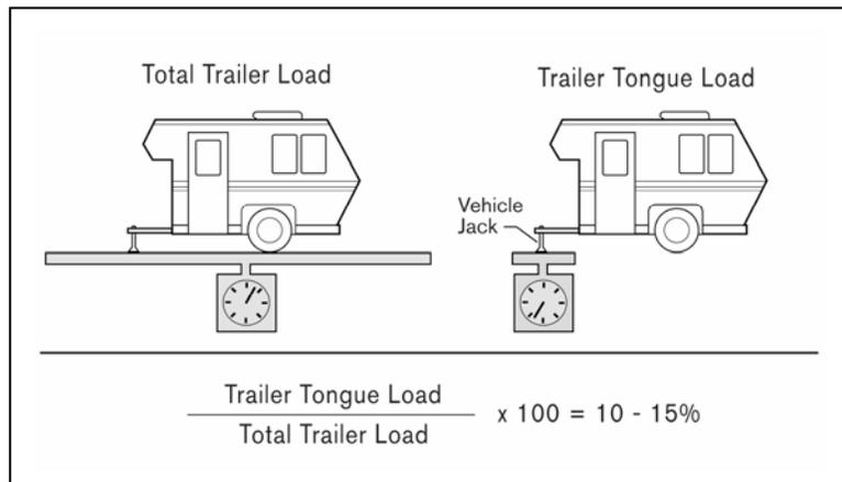
For proper handling, you must keep conventional trailer tongue load between 10-15% of the actual trailer weight, within the limits of the maximum trailer tongue load allowable.
