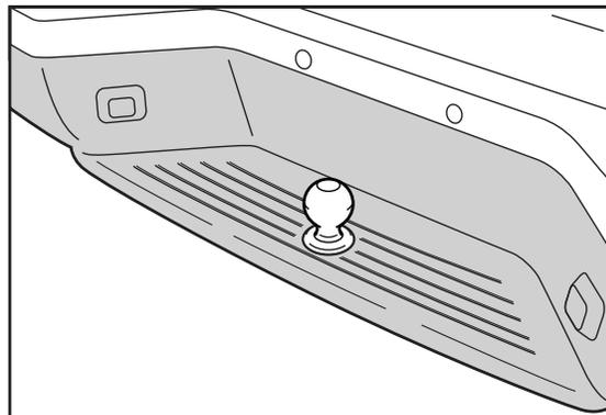
**Receiver Hitch** – A receiver hitch is bolted directly to the vehicle structure for added strength and durability. Nissan bolt-on receiver hitches are designed specifically for Nissan vehicles and include the necessary reinforcements, with ample clearance around bumpers, frame members, etc. These hitches allow for the removal of the ball mount when not towing.
