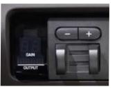
• Redesigned user-friendly display indicates gain, TBC output and trailer connection status, including disconnect alarm and message center warning
