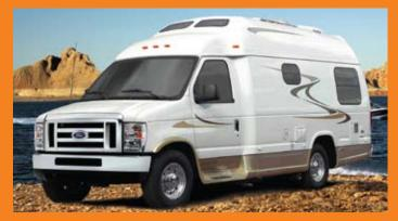
E-Series vans provide an excellent base unit for Class B campers. Converters make major modifications, including sleeping, kitchen and bathroom facilities, as well as 110-volt electrical hookup, fresh water storage and/or city water hookup. These custom conversions typically include a high roof that can provide greater comfort by allowing occupants to stand up inside. If a Class B van camper matches your recreational needs, make sure it starts out as a Ford E-Series van.
