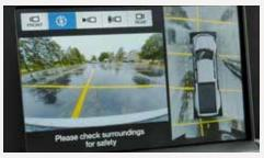
Trailer Reverse Guidance uses 3 cameras to provide multiple views of trailers, as well as steering guidance graphics, to assist with trailer maneuvers while in reverse
