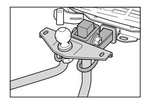
own an Armada, Frontier, Pathfinder, or Titan vehicle and plan to tow trailers with maximum weight over 5,000 lbs. This ball mount includes a  $2^{5}/_{16}$ " hitch ball rated for up to 10,000 lbs., and is available through your Nissan dealer for use with the optional tow package.
