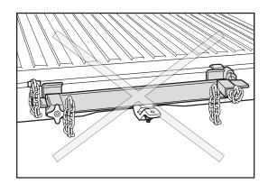
bumper and bodywork, and may possibly result in trailer separation during towing. Therefore, tow only with a permanent hitch.
