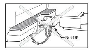
chains/cables when making a sharp turn, do not attach the chains/cables too close to the coupler. Consult your trailer manufacturer for the proper location of the chain/cable attachment to the trailer.
