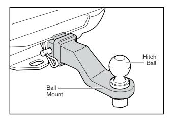
selected has the proper shank diameter and weight rating for the ball mount as well as the coupler on your trailer. Using a  $1^7/_8$ " hitch ball in a 2" coupler, for example, could result in the trailer separating from the tow vehicle.
