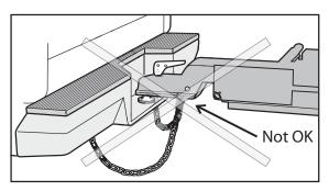
to the bumper and chains/cables when making a sharp turn, do not attach the chains/cables too close to the coupler. Consult your trailer manufacturer for the proper location of the chain/cable attachment to the trailer.
