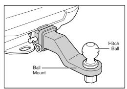
shank diameter and weight rating for the ball mount as well as the coupler on your trailer. Using a 1<sup>7</sup>/<sub>8</sub>" hitch ball in a 2" coupler, for example, could result in the trailer separating
